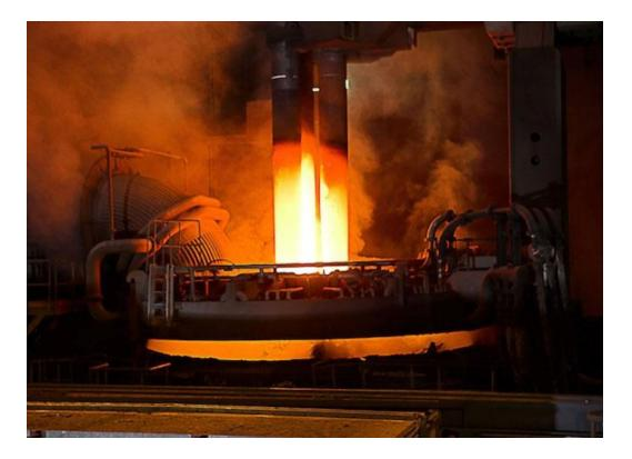
Graphite electrodes are used mainly in electric arc furnace steel production. Furthermore, coatings has been used on **graphite electrodes** since 1969 in these industries for steel melting, ranging from 5 tonnes to 185 tonnes capacity, using 200 ~ 600 mm diameter electrodes. Graphite electrodes are used for producing STEEL.
